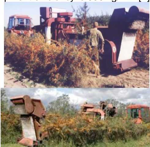
Figure 9 Mobile equipment for sea blackthorn separation [22, 23]
