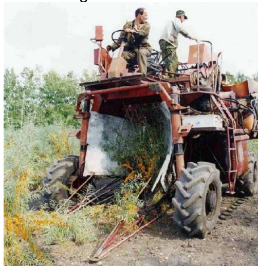
Figure 10 Canadian sea buckthorn harvesting self-propelled machine [8]
