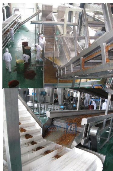
Figure 12. Technological line for seabuckthorn pre-processing [29]
