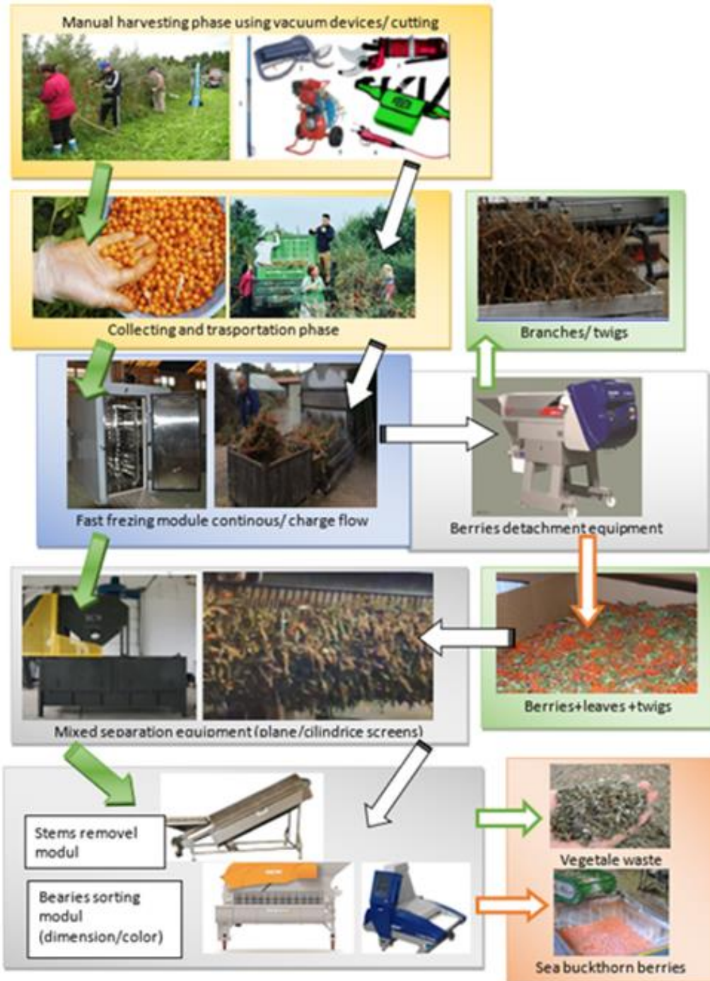
Figure 12 Block diagram of INMA technology to separate sea buckthorn berries [31]
