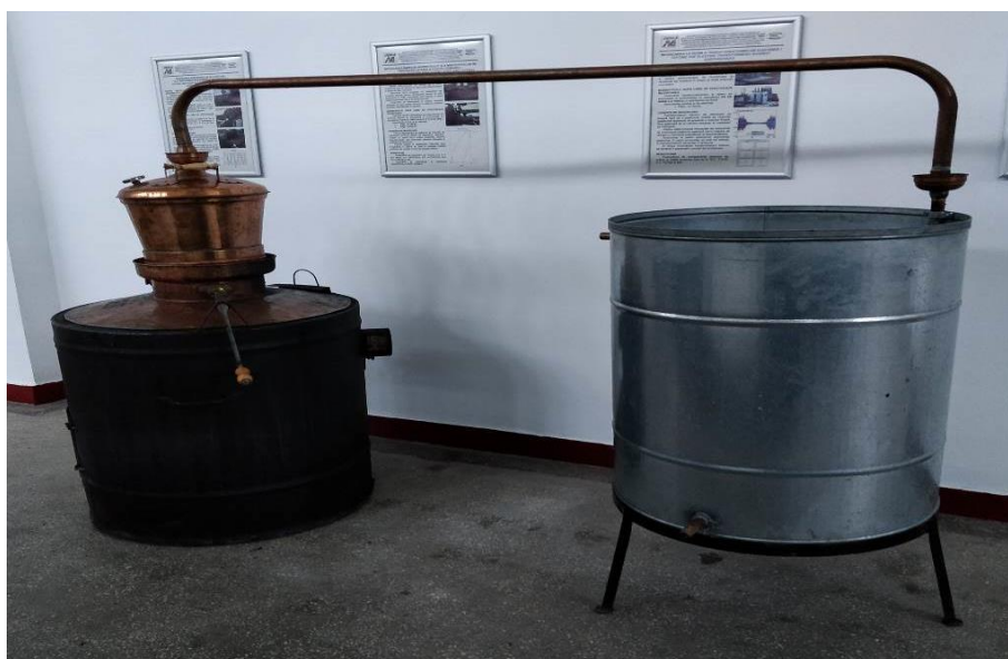
Fig. 3. Installation for distillation / obtaining raw alcohol (IOAB)
