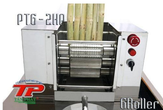
Fig.1. Instalation for obtaining juice from sugar sorghum stems [19]
