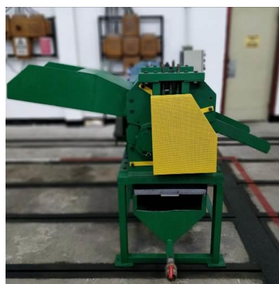
Fig. 7. Press used in experiments to obtain juice
