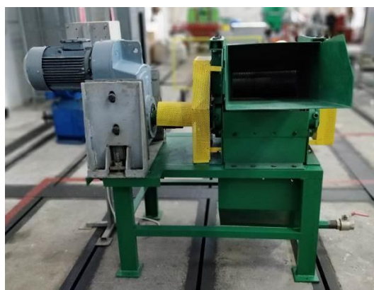
Fig. 7. Press used in experiments to obtain juice
