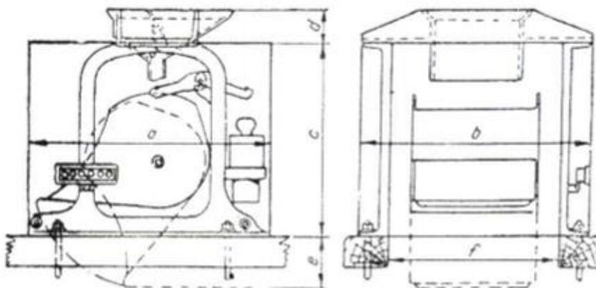
**Fig. 3. Schematic diagram of Chronos automatic scale [7]**
