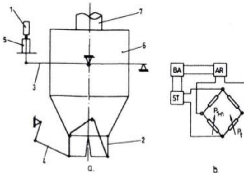
**Fig. 7. Schematic diagram of discontinuous bulk material dispenser [19]**
