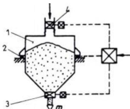
**Fig.5. Gravimetric discontinuous bulk dosing systems for bulk materials by addition of material [19]**
