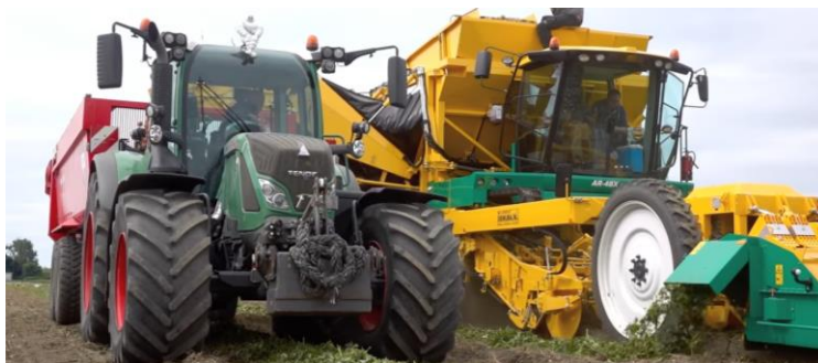
Figure 3 – Harvesting of the Jerusalem artichoke with self-propelled combine [4]
