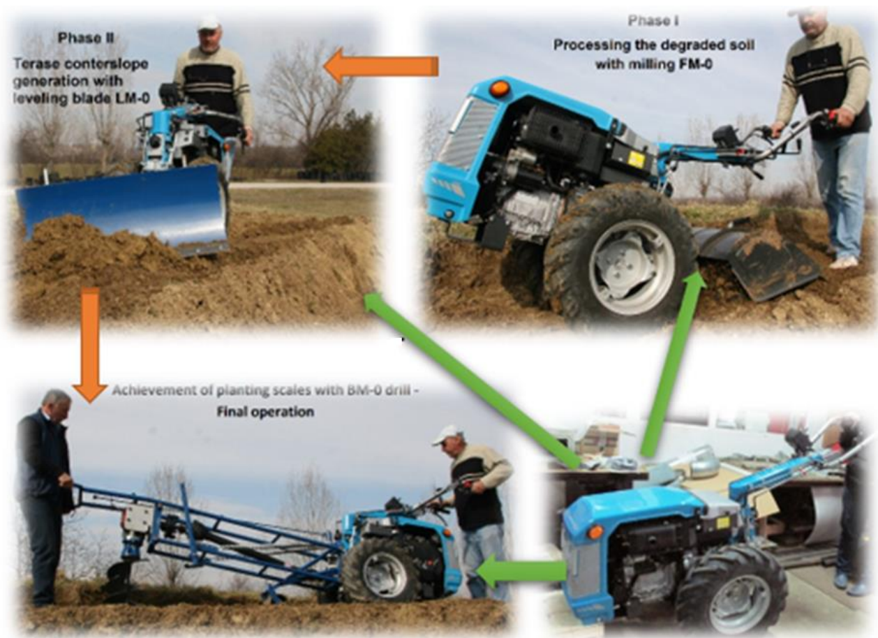
Figure 8 Experimental procedure during the working conditions on 25° counter-slope terraces
