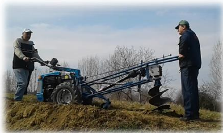
Figure 9 Experimental procedure to test the drilling equipment on 25° slope degraded terrain
