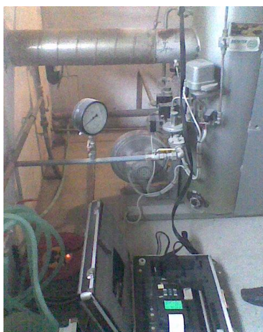
Figure 2: Mounting the devices and sensors required to measure the steam jet temperatures in the area of granulation mold
