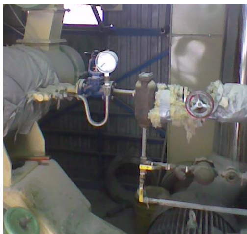
Figure 2: Mounting the devices and sensors required to measure the steam jet temperatures in the area of granulation mold
