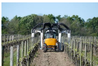
Fig. 14 – Ecoprotect spraying machine [16]
