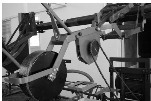
Fig. 3. Sowing section mounted on the bench
