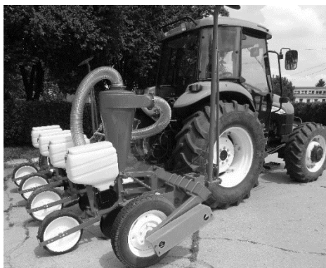
Figure 1. Eco-innovative system with "deflector" to reduce dust emissions when sowing
