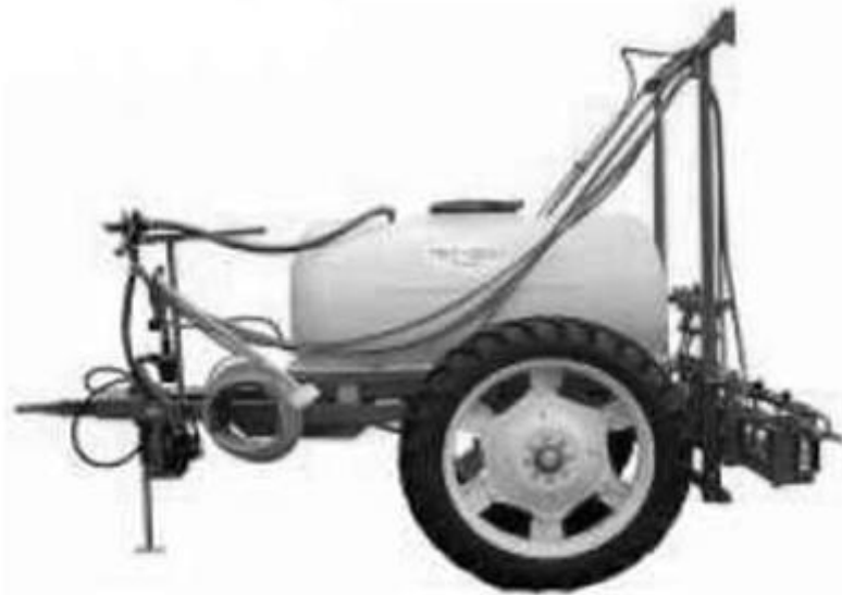
Fig. 2. Towed sprayer MET 1500 for the management of the herbicides, fungicides and liquid fertilizers in field crops.
