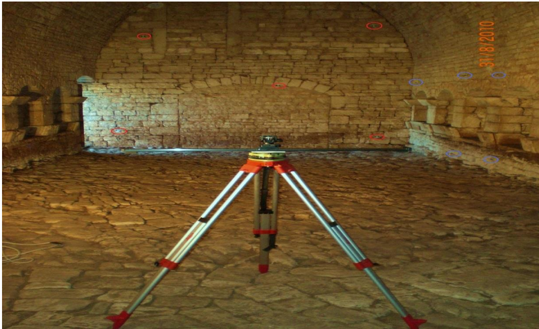
Figure 2 Photogrammetric landmarks. Red – landmarks on a wall; blue - landmarks on another wall of the same room
