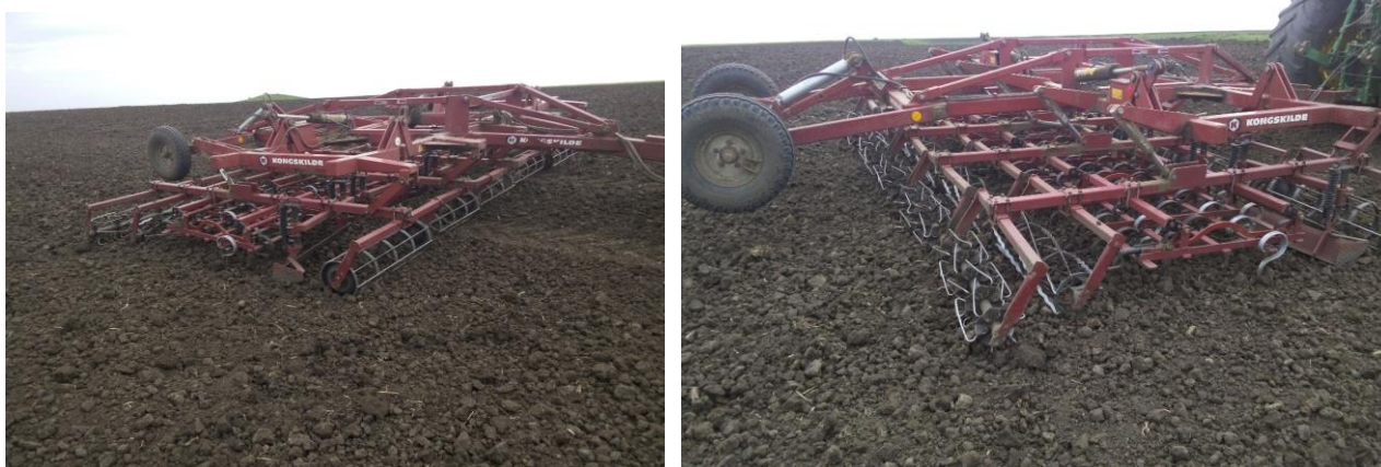
Fig.1. a) Set combiner achieved by KONGSKILDE company; b) The layout of the active components.
