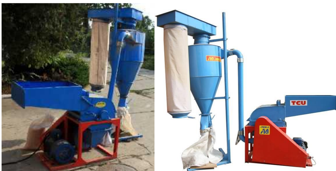
Fig. 1 - Vegetal waste mill (hammer mill) – MC 22
