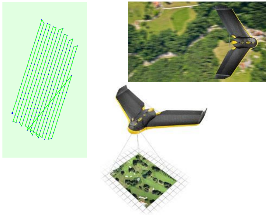
Figure 5 – Photographing of the test area along the line according to the defined flight plan
