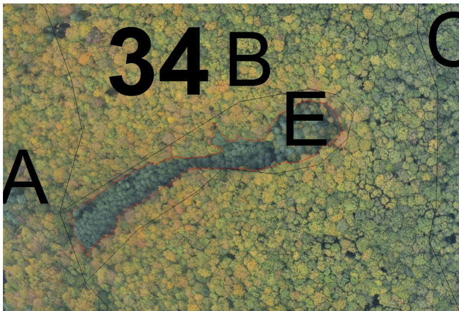
Figure 9 - Detail on the orthophotomap EB of Mihăești, with limits for 34E from GIS database (black line) and the vectorization lines from the ortophotomap (red line)
