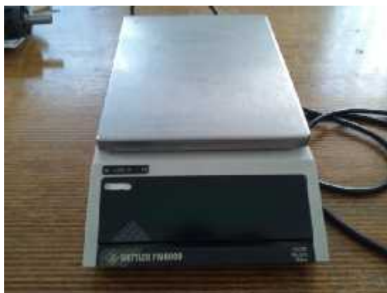
Fig. 4 – Precision electronic balance METTLER PM 6000
