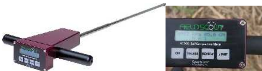
Fig. 6 – Digital electronic penetrometer with FIELDSCOUT SC 900 cone
