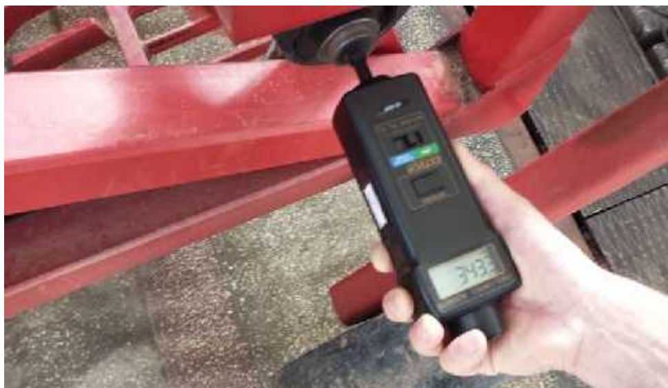
Fig. 5. Determining rotation frequency of separator driving shaft
