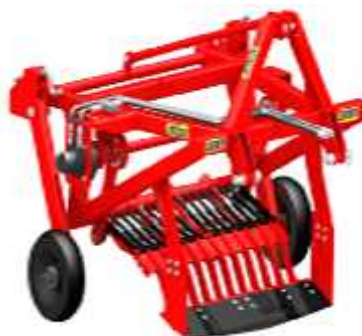
Fig. 1 – Equipment for harvesting the Miscanthus rhizomes [11]
