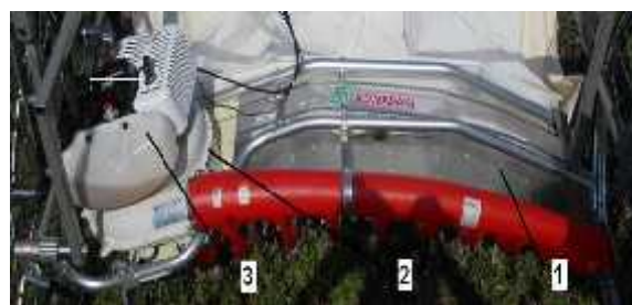
Figure 2 - The mower of the lavender harvesting equipment
