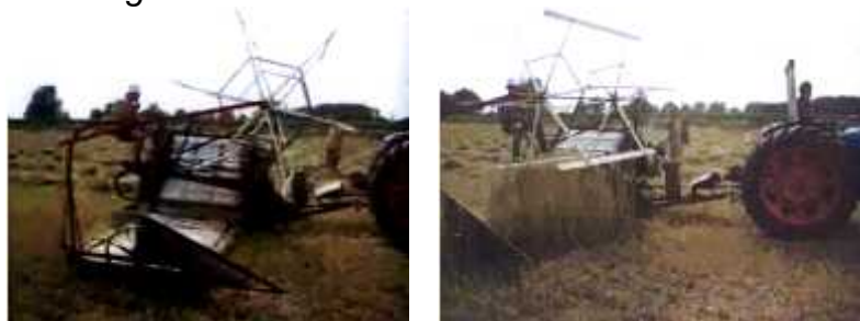
Fig. 8 – Tower reed harvesting machine [9]
