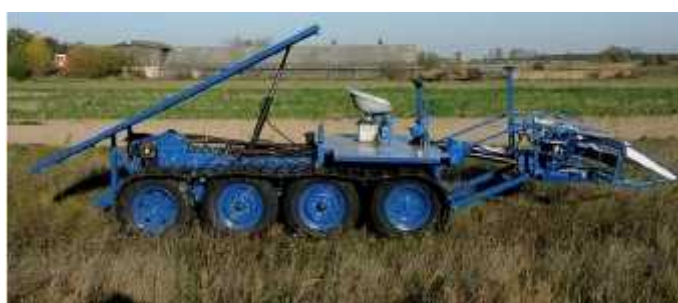
Fig. 4 - REEDA REED HARVESTER reed harvesting machine [5]
