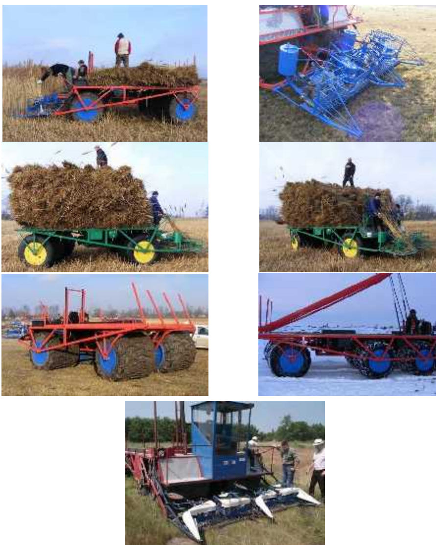
Fig. 2 - SEIGA 4x4; 6x6 reed harvesting machine [3]
