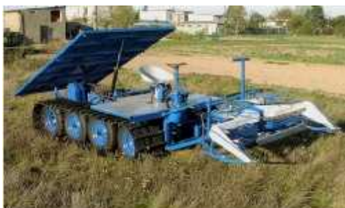
Fig. 4 - REEDA REED HARVESTER reed harvesting machine [5]
