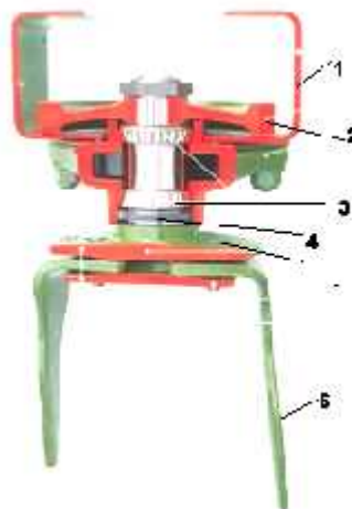
Fig.1 Construction and components of rotor blades 1-housing, 2-gear to drive the rotor, 3-bearing, 4-rotor flange; 5- uruburi6-knife
