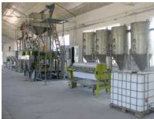
Fig. 3. The Installation for obtaining vegetable oils IEU 450 [2]
