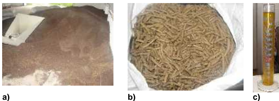
Fig. 4. Raw material and products obtained after cold pressing a – raw material (rapeseeds); b - pellets; c – vegetable oil;
