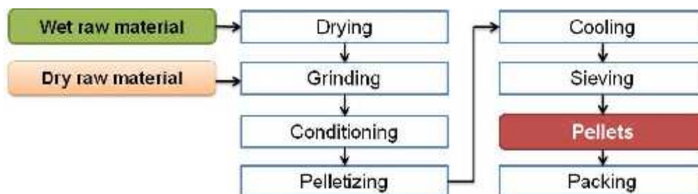
Fig. 1 – Pelletizing operation stages [16]
