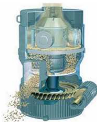
Fig. 4 – Operating principle of flat die pelletizing machines [5]
