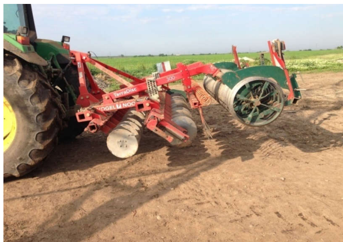
Fig.1. Independent disc harrow TERRADISC 300 manufactured by the company Vogel & Noot.
