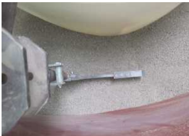
Fig. 7. Chisel type knife mounted on experimental stand
