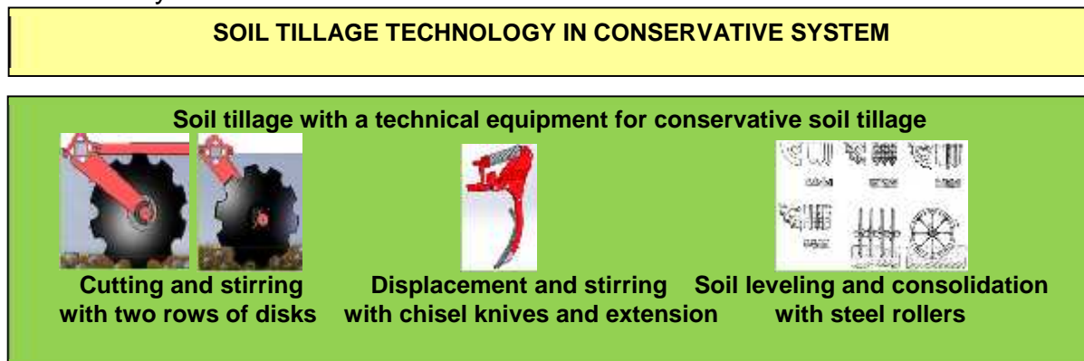
Fig. 2. Diagram of the technological flow for soil tillage in the conservative system
