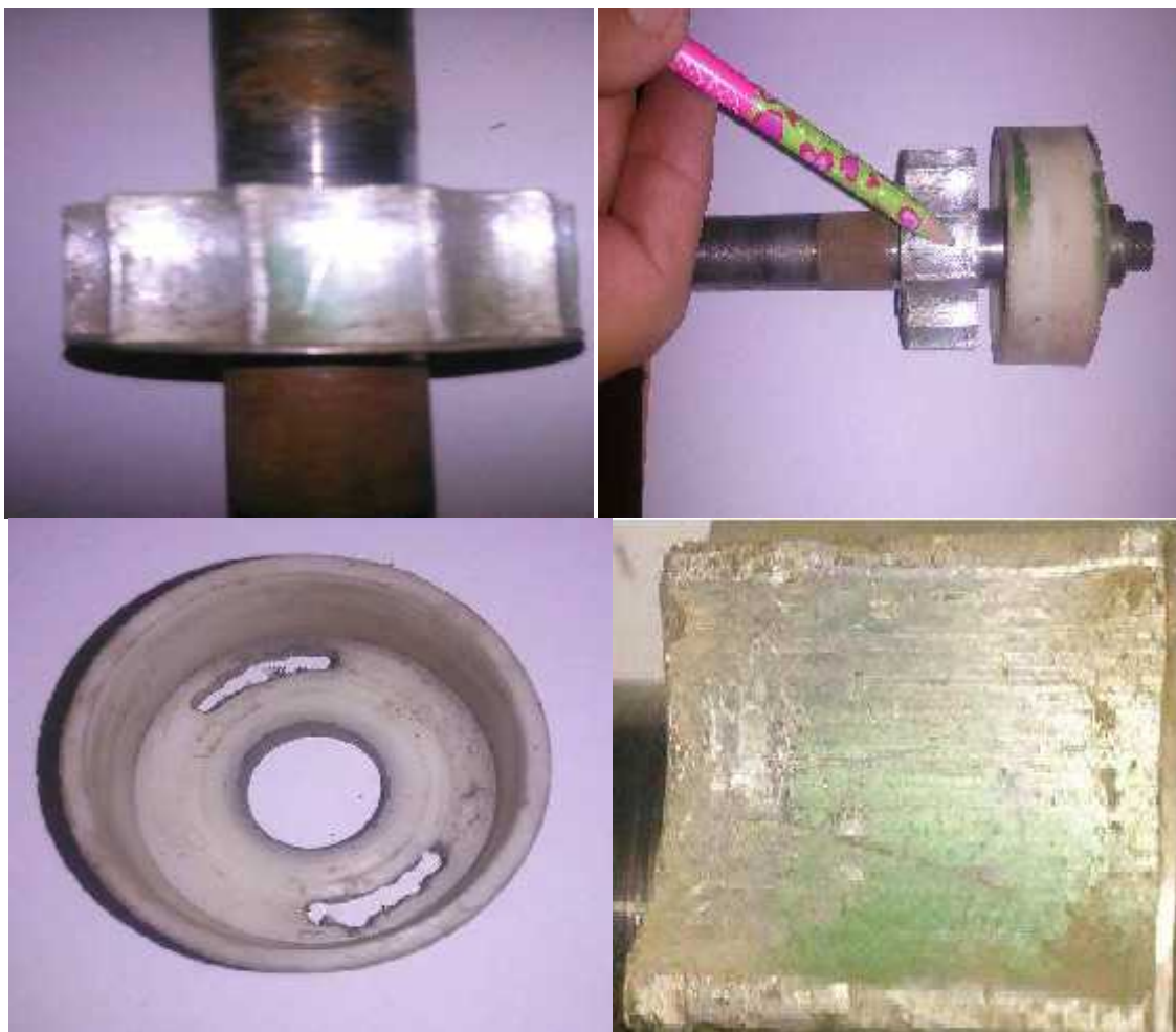
Fig. 2 - Distributor used in the construction of INMA drill
