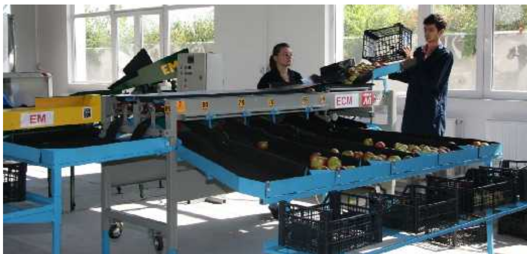
Fig.5 - Testing sorting equipment by dimension–working process aspect
