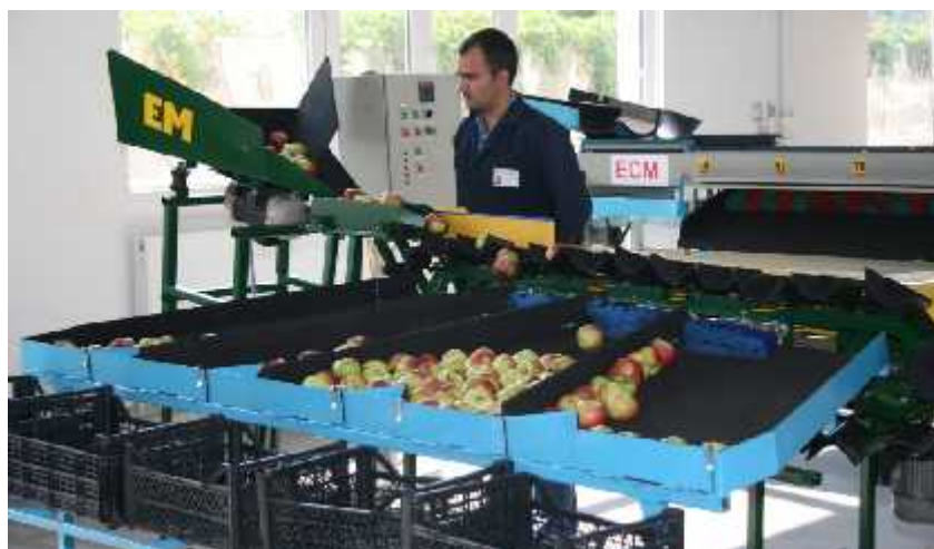
Fig.6 - Testing sorting equipment by weight–working process aspect
