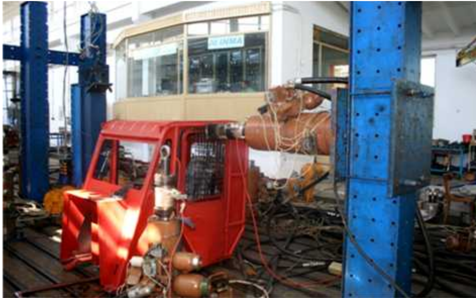
Fig. 3 - Mounting performed on "Hydropulse" facility for applying lateral loads
