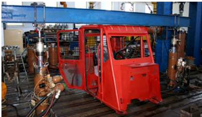
Fig.2 - Mounting performed on "Hydropulse" facility in case of frontal crushing
