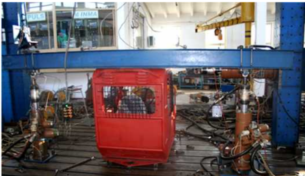
Fig. 4 - Mounting on "Hydropulse" facility for testing the cabin of TAF - 690 tractor in case of rear crushing
