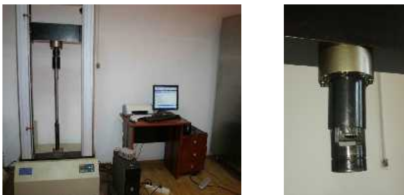
Fig. 1 - Installation for biomass compaction at reduced scale
