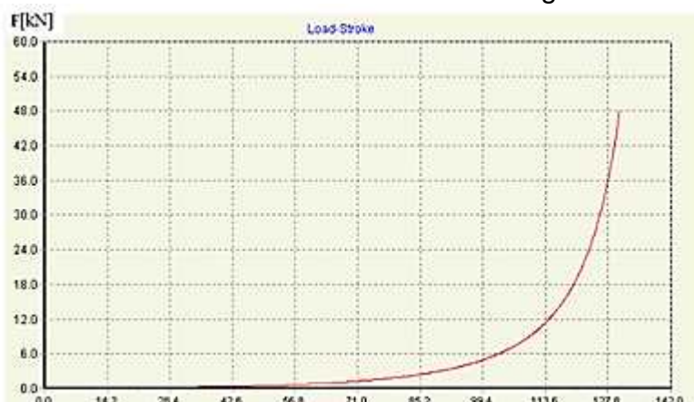
Fig. 3 – Densification force-deformation curve
