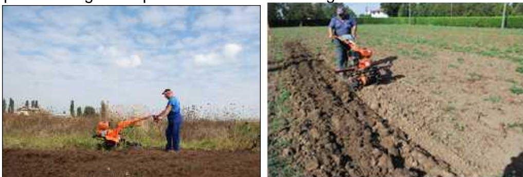
Fig. 1 – Tiller M7,5 in aggregate with cu reversible plow PR1 – during the experiments-
