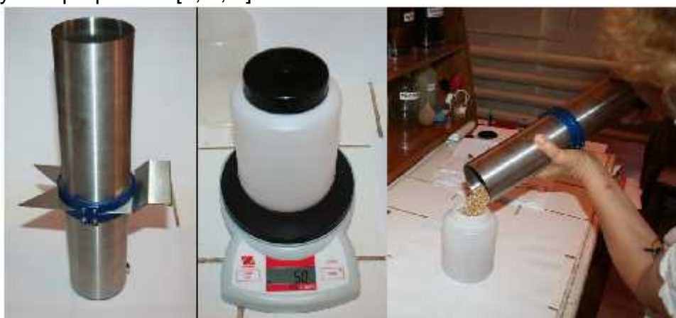
Fig.2. Determining the hectoliter weight
