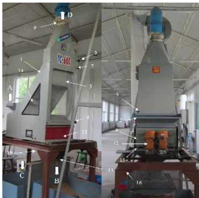
Fig. 1. Diagram for the equipment Combined Separator TC 600:
