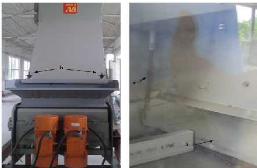
Fig.4. the system for adjusting the seed flow rate: a. damper plate; b. device for adjusting the feed rate; c. traction spring
