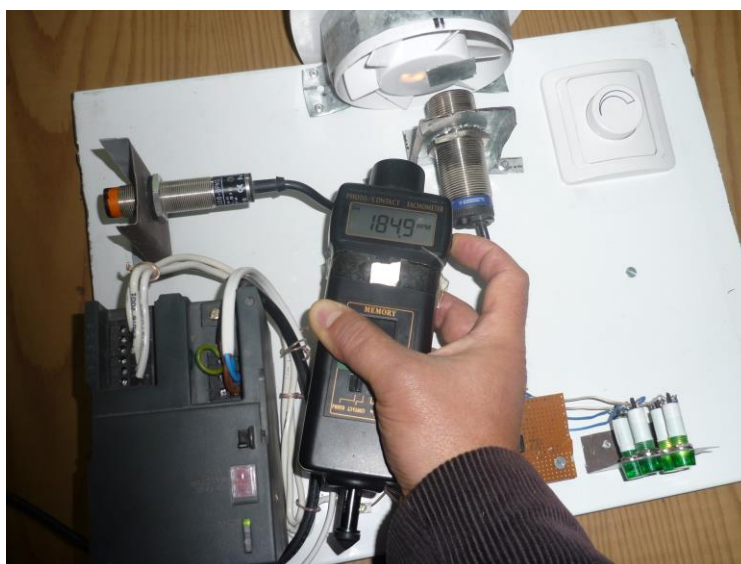
Figure 6: The usage of the EBRO DT-2236 electrical tachometer to determine the rotation of the metallic band attached to the cylinder
