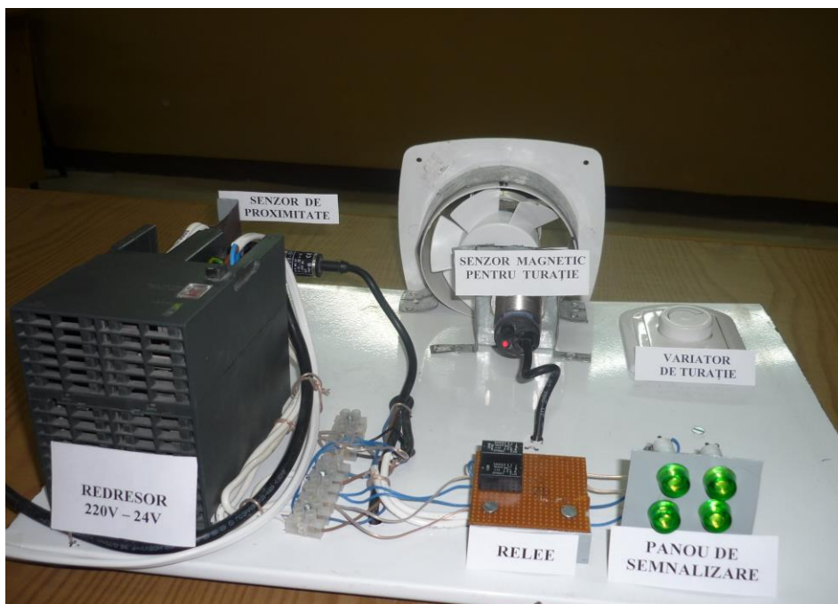
Figure 5: The electrical assembly used to study the function of the 2 metallic sensors
