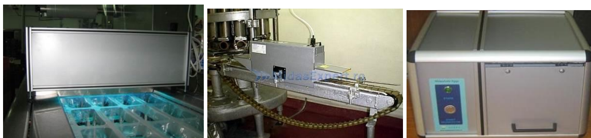
Fig. 8 – Equipment for disinfection of packaging and products MidasAnAir SU Packaging, MidasAnAir SU Conveyor and MidasAnAir Eggs [20]
