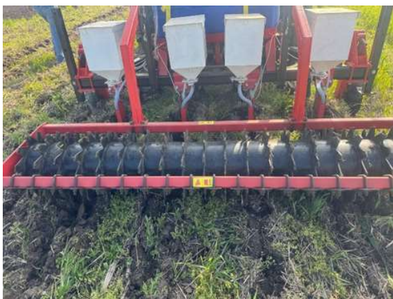
Figure 2. Scarifier equipped with equipment for inoculating microorganisms biostimulator into the soil
