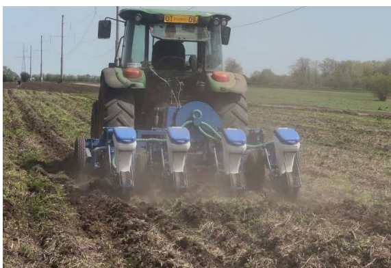
Figure 3. Precision seed drills for direct sowing in uncultivated soil
