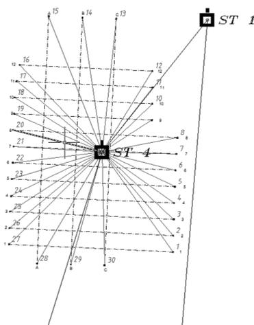
Figure 5. The lay-out plan of the leading marks
