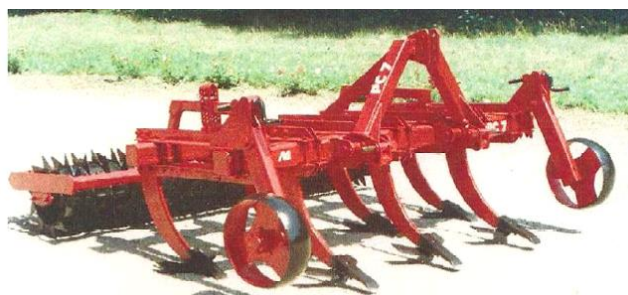
Fig. 8 – Equipment with 7 loosening bodies EA7 (PC7 chisel plow), fitted with toothed harrow [3]
