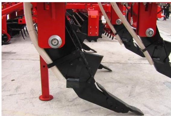
Fig. 2 – Active body of DECUM technical equipment [2]
