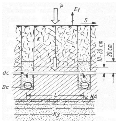
**Figure 8** - The effect of deep soil loosening on land with hard permeabil clay layer of large thickness
