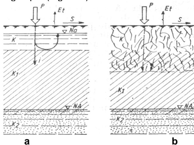
**Figure 7** – The effect of deep soil loosening on land with hard permeabil clay layer located at small depth
