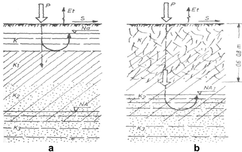
**Figure 6** – The effect of deep soil loosening on land with hard permeabil clay layer located at small depth
