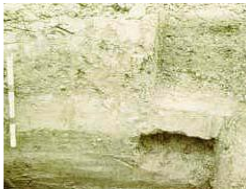
Fig. 3 - Example of hardpan
