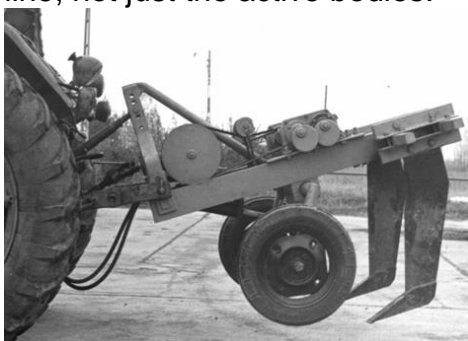
Fig. 13 - Subsolier vibrator SV-2, cu mase rotative neechilibrate [3]
