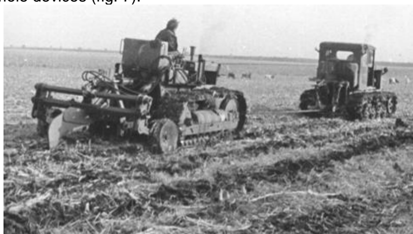
Fig. 7 – Loosening equipment MID-02 with mole device
