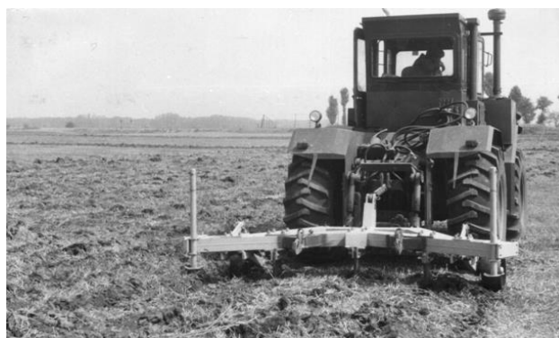
Fig. 11 - Mounted deep loosening equipment SP-3 (5) at work [1]
