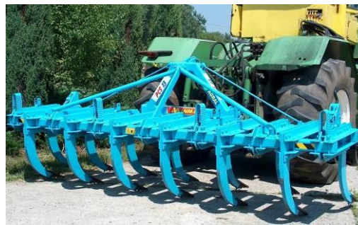
Fig. 16 - Chisel plow and deep loosening equipment PC13-0S [1]
