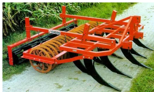
Fig. 32 - Everest deep loosening equipment Garron LT - 9K - 9K [16]
