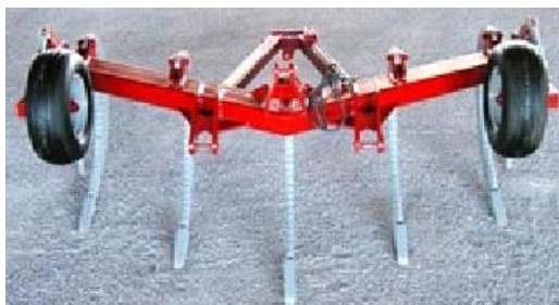
Fig. 28 - Deep loosening equipment DWK 250 / DWK 270 [13]
