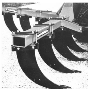
Fig. 9 - Deep loosening equipment with 7 bodies / 11 active bodies with curved supports [4]
