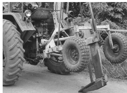
Fig. 11 - Deep loosening equipment with oscillating working body [5]
