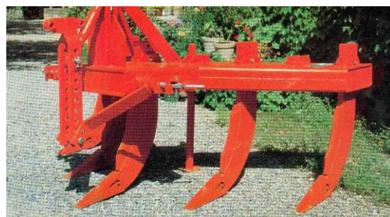
Fig. 27 - Scarifier for deep soil loosening equipped with rigid bodies [12]
