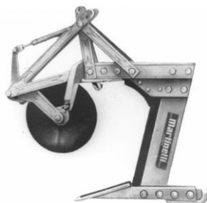
Fig. 5 - Deep loosening equipment AP-1, with a single active body [1]
