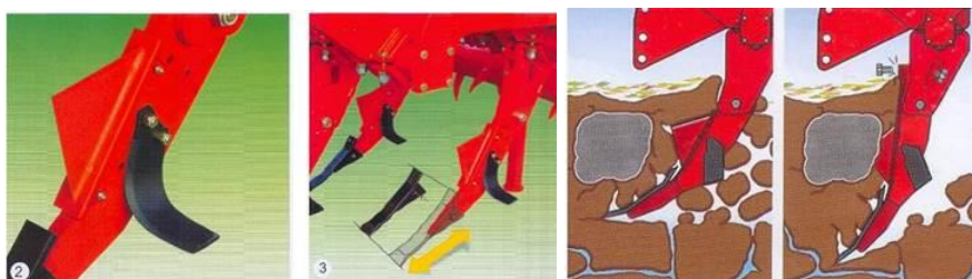
Fig. 16 - Active bodies deep loosening of soil [8]
