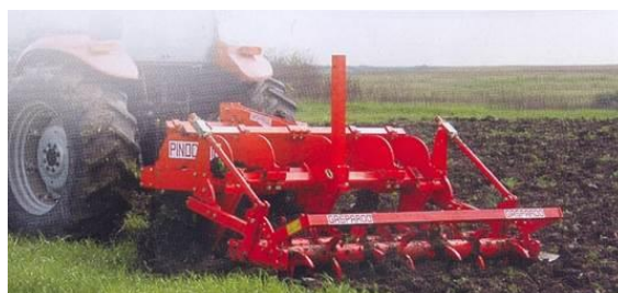
Fig. 18 - Deep loosening equipment PINOCCHIO [8]
