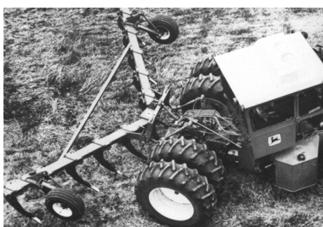
Fig. 9 - Deep loosening equipment with 7 bodies / 11 active bodies with curved supports [4]
