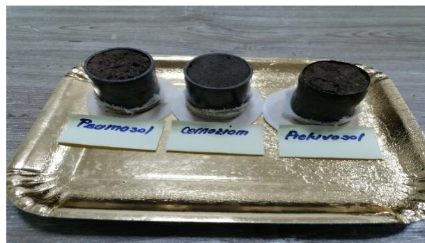
Figure1. Determination of soil permeability
