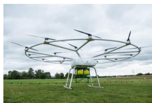
b) giant spray drone (200 kg payload)
