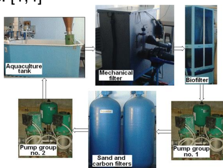
Fig.3. Technological structure of the recirculation system [4]
