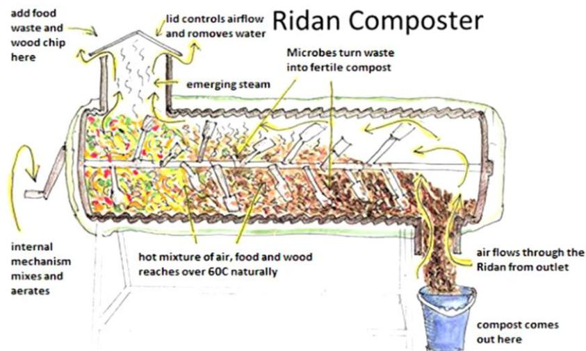
**Figure 9. Ridan Composter**, (Source: <http://www.ecovrs.com/en/products/in-vessel-composting/ridan-composter/>)
