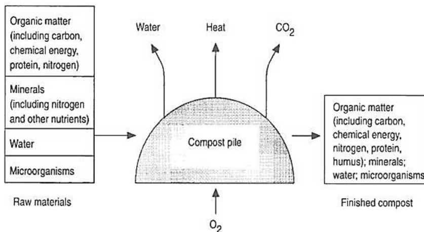
Figure 2. The composting process, (Source: <https://content.ces.ncsu.edu/large-scale-organic-materials-composting>)
