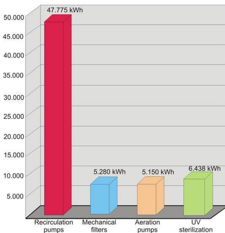
Figure 1. Graph of the annual electricity consumption for the treatment and circulation of water from a recirculating aquaculture system
