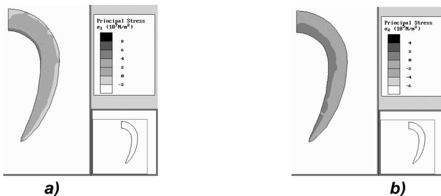
**Fig. 4. a) Main stresses  $\sigma_1$ , b) Main stresses  $\sigma_2$**
