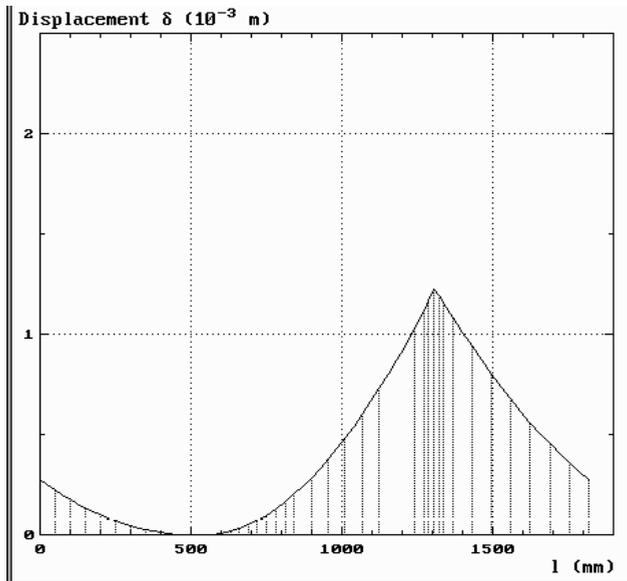
**Fig. 6. Variation of nodal displacements along the entire contour of the stilt**
