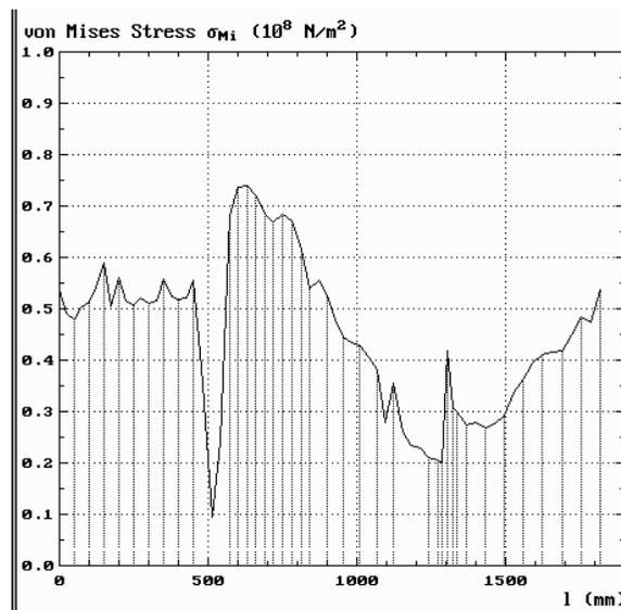
**Fig. 7. Variation of equivalent stresses along the entire contour of the stilt**
