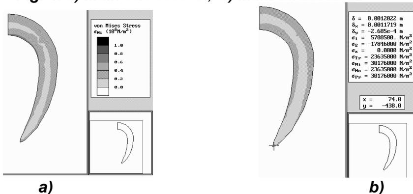
**Fig. 5. a) von Mises equivalent stresses, b) The set of results for the point in the Figure**
