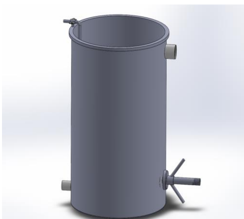
Fig.5. Cooling (condensation) vessel
