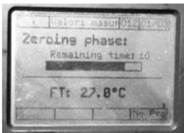
Figure 1 - Calibration and setting of measurement parameters at TESTO 350 M/XL
