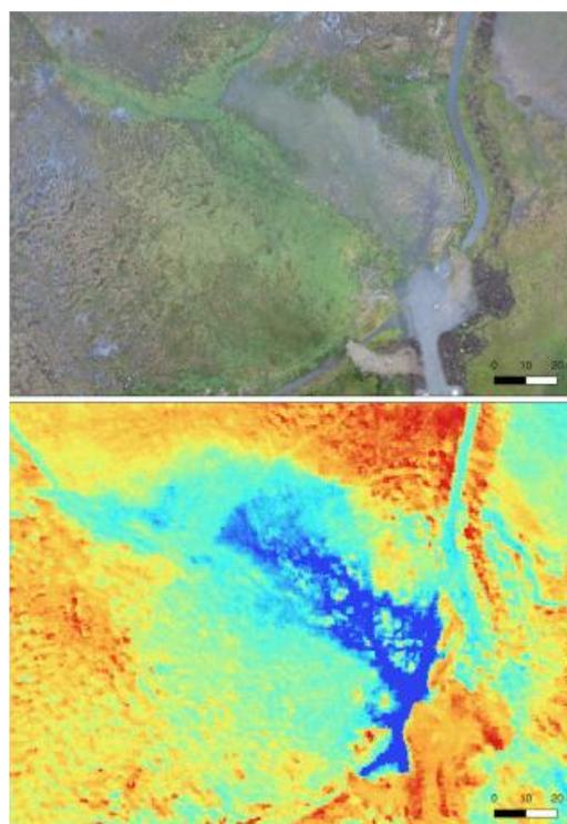
*Figure 7: Drone-based normal colour photos (top) and TIR images (bottom) of wetlands. Temperature differences in the TIR images show possible groundwater upwelling as indicated by colder*
