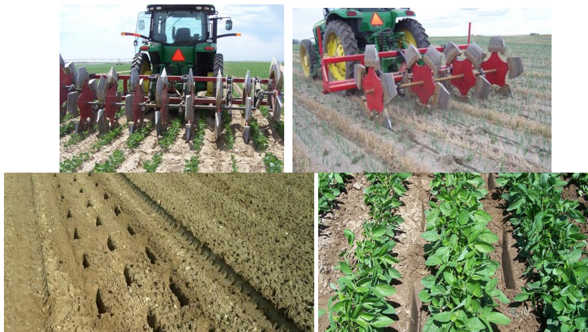
Fig.3. Pocket Pitter equipment for making micro-tanks in narrow-row cultures [11]
